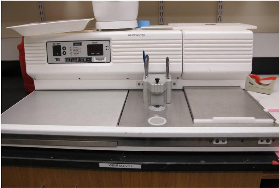
Warmer and hot plate for Embedding. See forceps are inserted into the place which will be heated when turn on.
