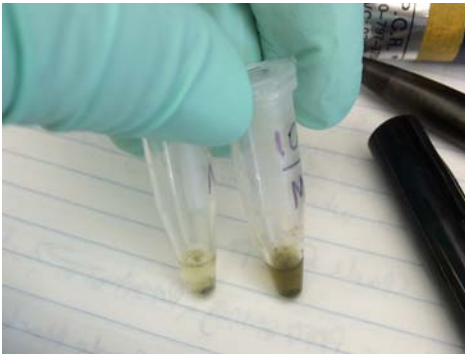
Figure 6. Example of chlorophyll and lipids that will not go back into solution after resuspension in MS extraction buffer.
